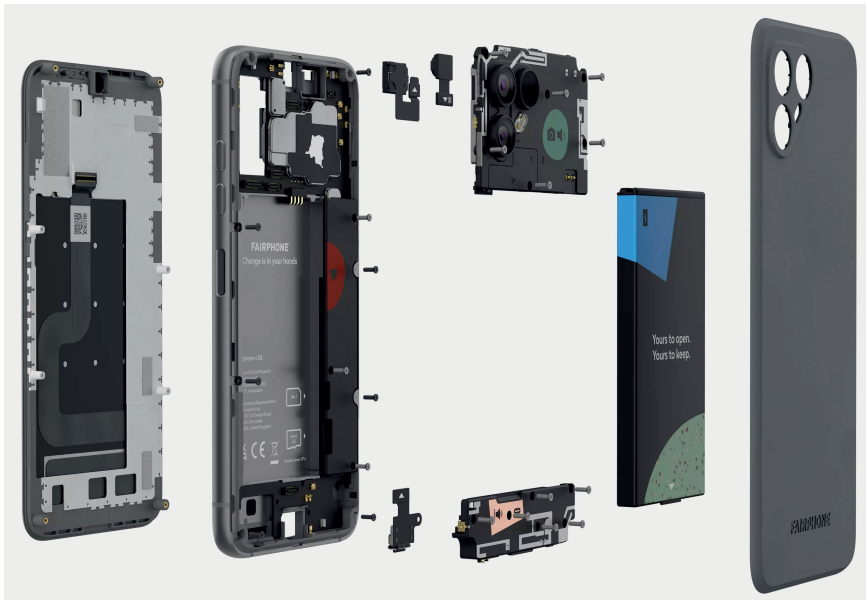
Fig. 3. The modular design simplifies the repair and recycling of the smartphone “Fairphone”.
